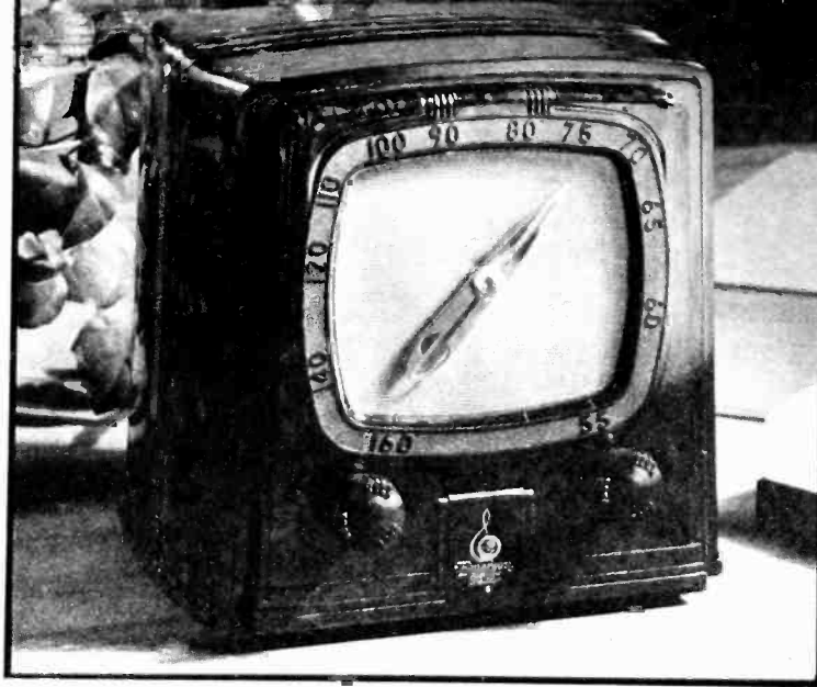
Two views of the Emerson midget receiver with dial surrounding the speaker grille. The dark cabinet is of mottled Durez, while the ivory housing is of Beetleware. These illustrations show the variety which may be obtained through the use of plastics of various colors and compositions
